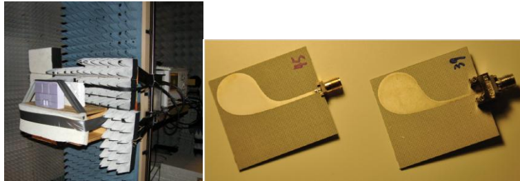
Figure 2 — SAR measurement setup and antipodal Vivaldi antenna
